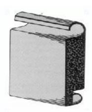
When an application requires weather protection the R&S "Thermal Guard" steel rolling service door is the right choice. Constructed using laid-in-place polyurethane insulation the curtain is an effective barrier against the elements. Rain, dust and wind are kept at bay by vinyl weatherstripping at the footpiece, guides and hood. Designed for sizes up to 30' wide and 28' high with a minimum 22 gauge exterior slat and a 24 gauge back slat these doors are constructed to stand against the elements.
